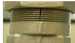
Crack on Parting Line
